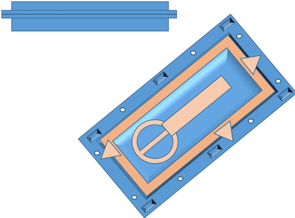
This leaves you with a two part mould with an accurate register to allow assembly – a series of drilled holes allows the mould to be bolted securely together.
