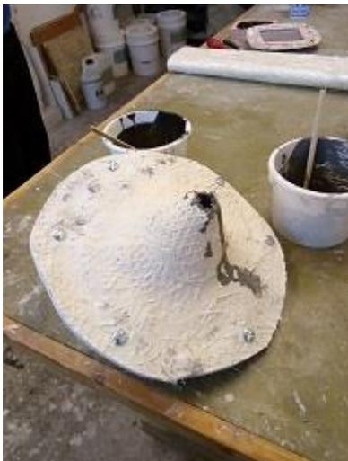
Jesmonite AC 300 laminated 2 part mould jacket over a silicone mould for slush moulded polyester ball.
